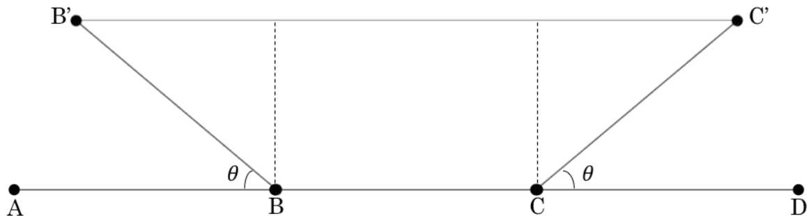
Figure 1: Geometry used to prove that only 1, 2, 3, 4, and 6 -fold rotation axes are permissible
